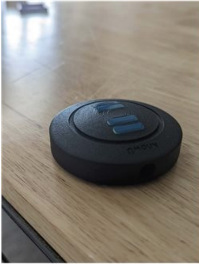
This is a 3D printed prototype of the KnowU for internal testing.
